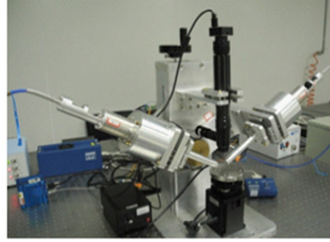
Figure 1. Principle and prototype of the dual rotating-compensator Mueller matrix ellipsometer.
