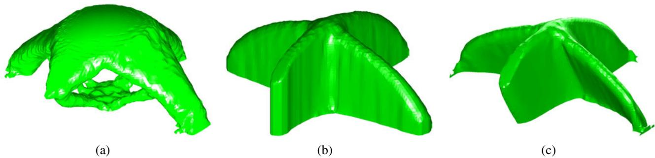
**Fig. 7** The optimal structures. **a** without considering molding constraint, the compliance is 258; **b** with molding constraint (parting direction is pre-selected to be along z axis, parting surface is pre-selected to be the bottom of the spherical cap), the compliance is
