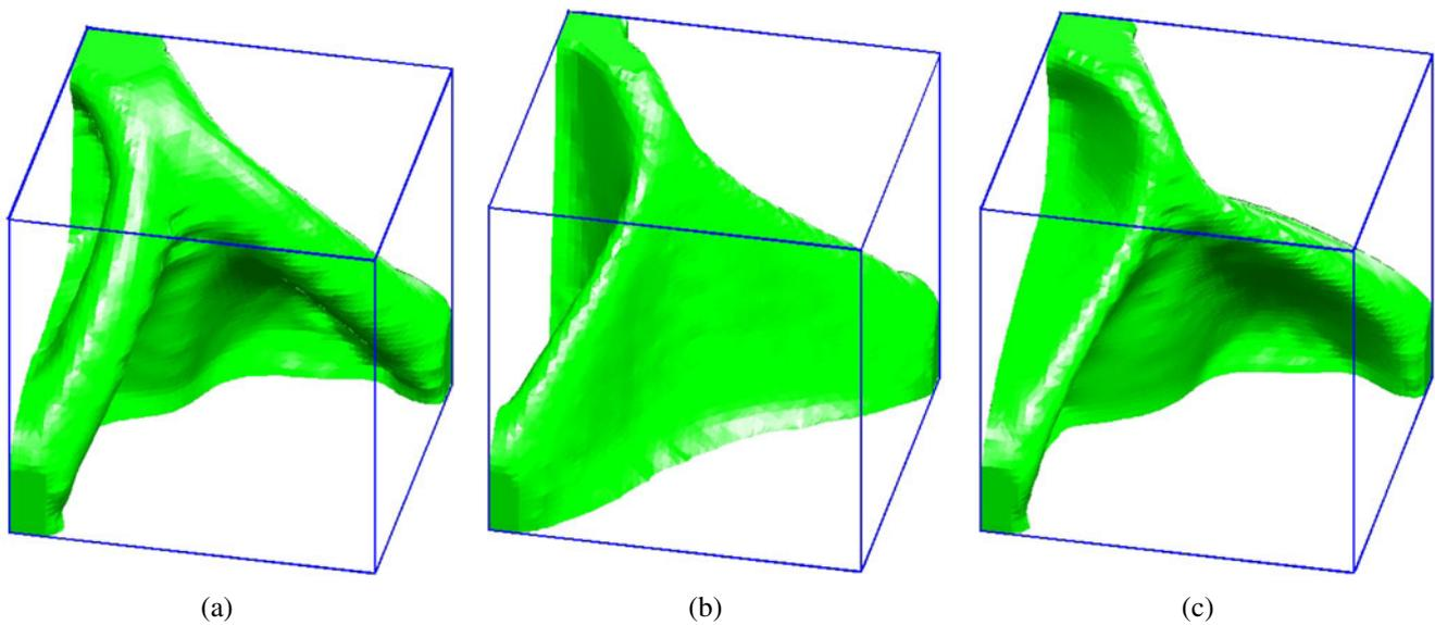
**Fig. 4** The optimal structures. **a** without considering molding constraint, the compliance is 452; **b** with molding constraint (parting direction is pre-selected to be along z axis, parting surface is pre-selected to be the bottom of the cube), the compliance is 502; **c** with
