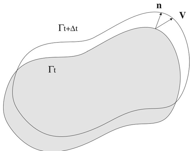
**Fig. 1** The velocity and the propagation of a boundary
