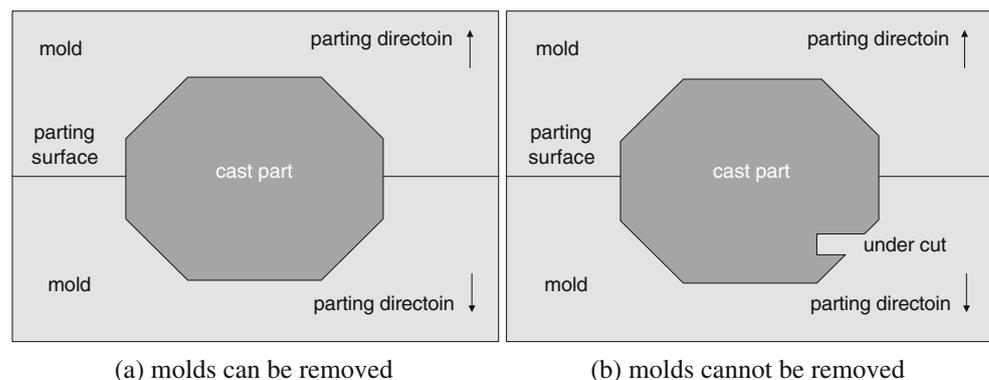
it reduces the costs of mold fabrication and the complexity of mold operation.
