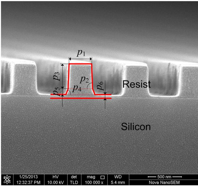
FIG. 1. X-SEM image and geometric model of the investigated nanoimprinted grating structure.
