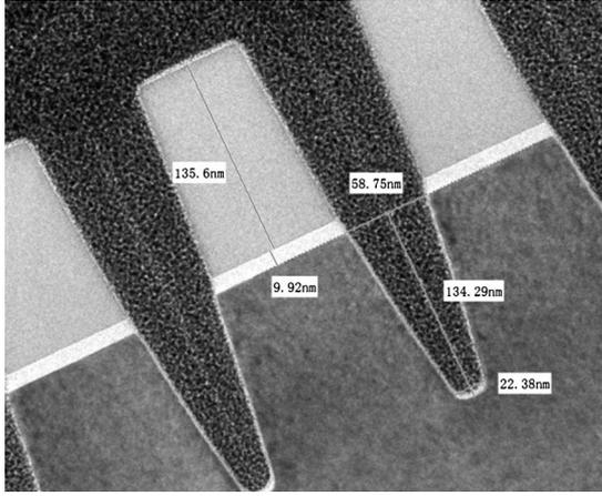
Fig. 1. Cross-section TEM image of the investigated deep-etched multilayer grating, which consists of Si, SiO<sub>2</sub>, and Si<sub>3</sub>N<sub>4</sub> trapezoidal gratings from bottom to top.
