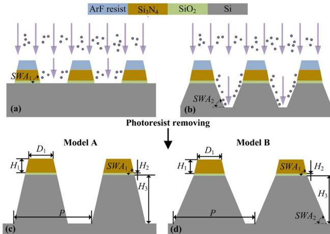
Fig. 2. Etching for (a) Si<sub>3</sub>N<sub>4</sub>/SiO<sub>2</sub> layers and (b) Si substrate in one etching procedure, and the two possible profile models of (c) uniform SWA and (d) nonuniform SWA after photoresist removing, respectively.
