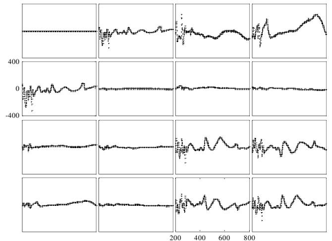
**Fig. 3. Weighted fitting differences of Mueller matrix elements. The Mueller matrix elements are normalized to  $m_{11}$ . The horizontal axes, varying from 200 to 800 nm with an increment of 1 nm, denote the wavelengths; the vertical axes, varying from  $-400$  to  $400$ , denote the associate weighted fitting differences.**
