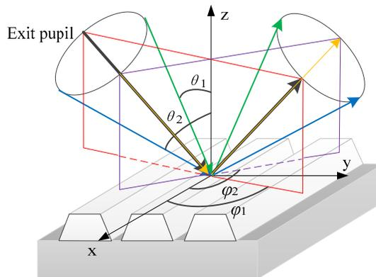
Figure 1. The variation of the incidence angle and azimuthal angle affected by NA.
