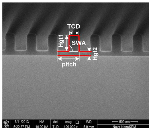
Figure 5. SEM cross-section image of the investigated photoresist grating.
