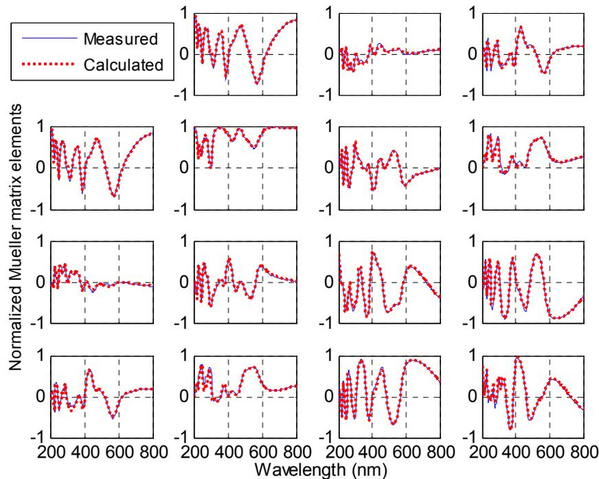
Figure 8. Example of the measured (red dash lines) and calculated (blue solid lines) spectra of normalized Mueller matrices for the investigated photoresist grating at the azimuthal angle of  $60^\circ$  and incidence angle of  $65^\circ$  by performing the correction method.
