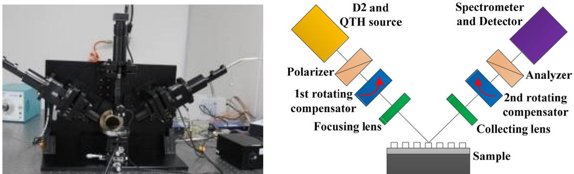
Figure 4. System setup and basic scheme of the dual-rotating compensator Mueller matrix ellipsometer.
