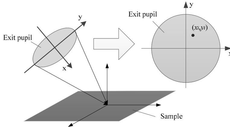
Figure 2. The corresponding incidence angle and azimuthal angle to the position in the exit pupil.
