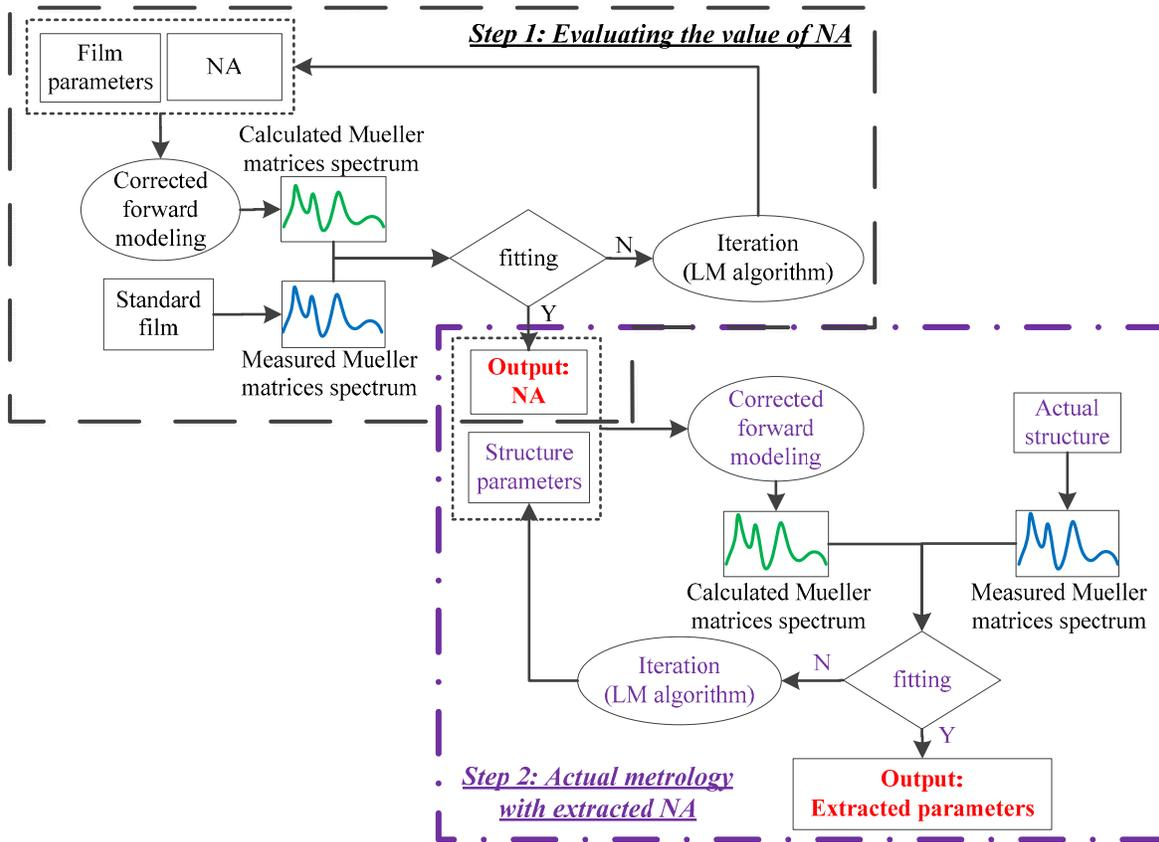
Figure 3. Flowchart of parameter extraction with corrected forward modeling.
