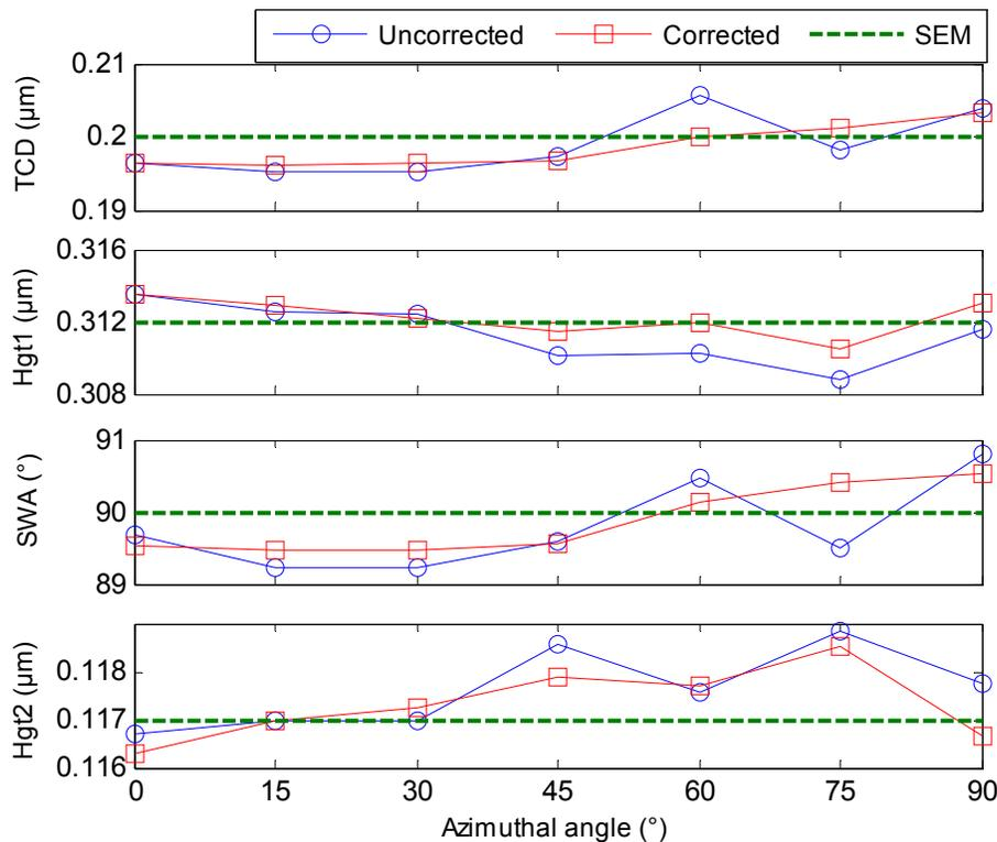
Figure 6. Comparison between the CDs measured by SEM and exacted from the same measured data by MMP at different azimuthal angle with and without the correction.
