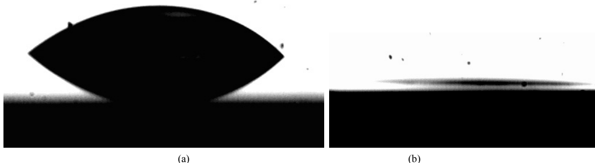
Figure 4. Contact angle of (a) untreated surface was 40.46° and (b) activated one was 3.76°
