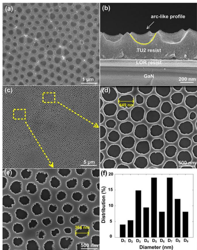
Fig. 3. (a) Top and (b) cross-sectional SEM images of the imprinted resist. (c)–(e) are PCLS patterned p-GaN. (f) Size distribution of the nanopores on p-GaN. The domain of 126–449 nm is divided into nine equal-interval parts ( $D_1 - D_9$ ) with the increment of 35.9 nm.
