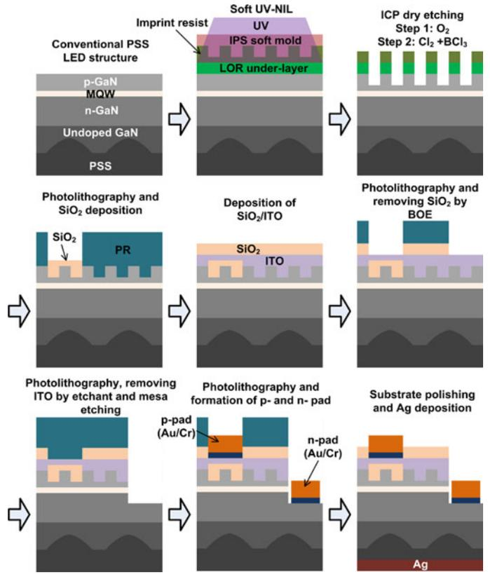
Fig. 1. The fabrication process of the patterned LED device with PCLS on the p-GaN layer of the GaN-based LED by using NIL and etching processes.
