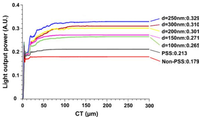
Fig. 7. FDTD simulation results on light extraction of the conventional LED, the LED on the PSS and the PCLS patterned LED with PSS. The thickness of p-GaN is 400 nm for  $d = 200, 250,$  and  $300$  nm.
