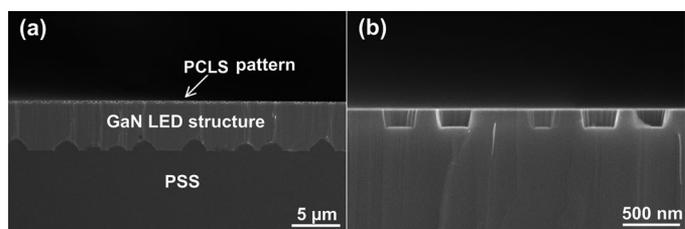
Fig. 4. (a) Low and (b) high magnitude SEM images of the LED device with the PCLS pattern times are 2 h and 10 s, respectively.
