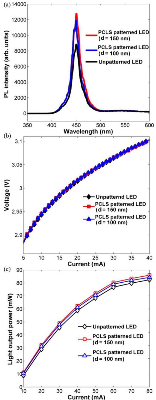
Fig. 5. (a) PL intensity versus wavelength for un-patterned LED device and the patterned LED devices with PCLS patterns of 100 and 150 nm in depth. (b)  $I-V$  characteristics of the un-patterned LED device and LED devices with PCLS patterns. (c) Light output power versus injection current for the un-patterned LED device and the patterned devices with PCLS. All LED devices are fabricated on the PSS.
