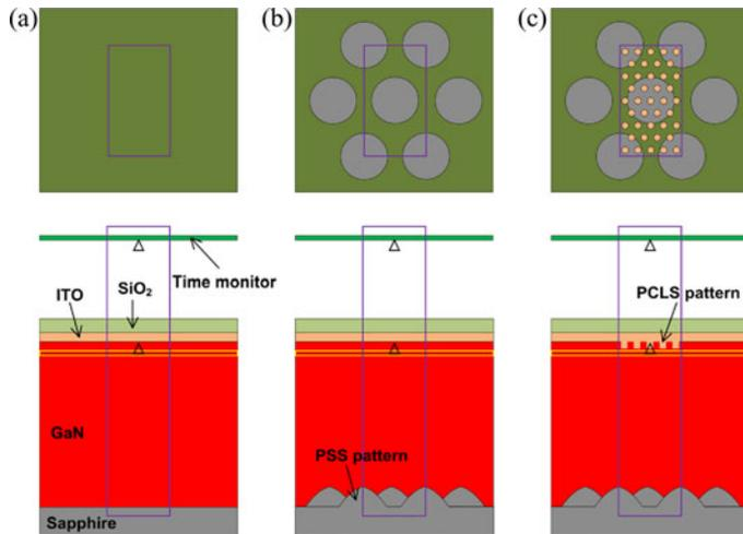
Fig. 6. Simplified FDTD simulation designs of (a) the conventional LED, (b) the LED with PSS and (c) the LED with PCLS patterns and PSS.
