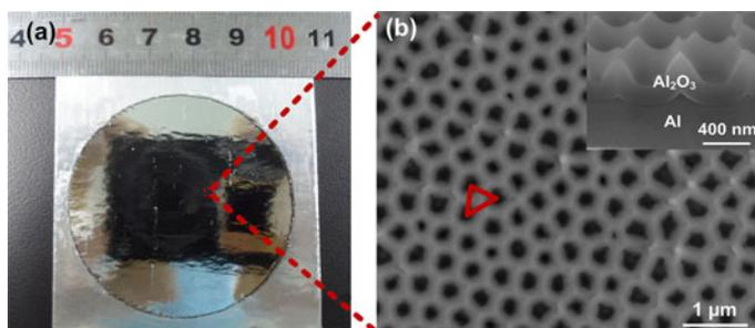
Fig. 2. (a) Photography and (b) SEM images of the 2 in AAO. The AAO is fabricated in a 1 wt%  $\text{H}_3\text{PO}_4$  + 0.01M  $\text{Al}_2(\text{C}_2\text{O}_4)_3$  mixture solution under the temperature of 5 °C and the voltage of 185 V. The first and second anodization times are 2 h and 10 s, respectively.
