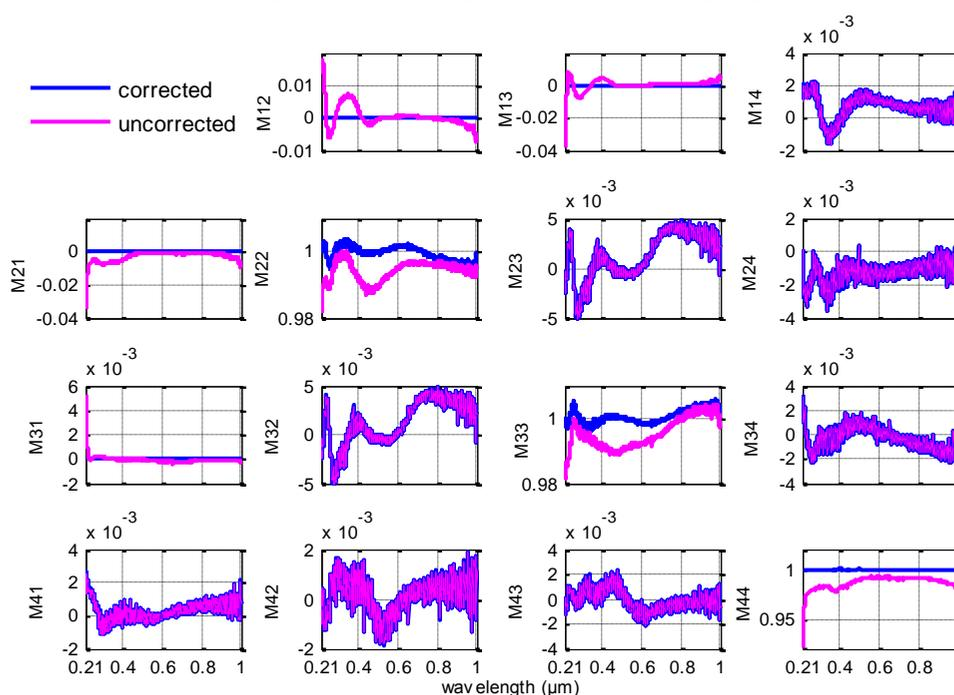
Fig. 3. Comparison between the Mueller matrix calculated from the same measured data by the MMP with and without the correction.
