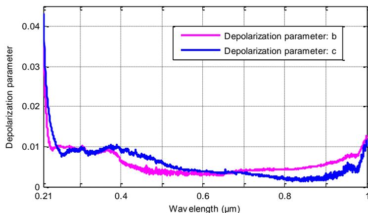
Fig. 2. Depolarization parameters of the compensators in the dual rotating-compensator MMP.
