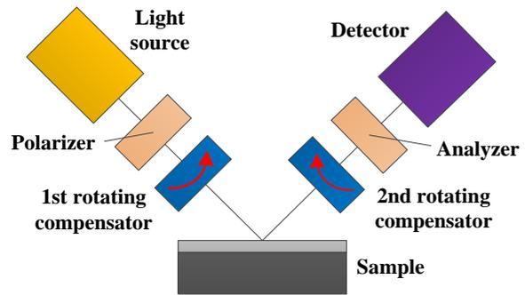
Fig. 1. Home-made dual rotating-compensator MMP.
