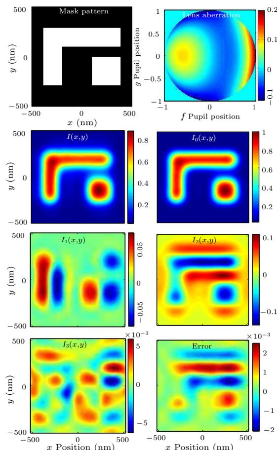
Fig. 3. Fast evaluation of aberration-induced intensity distributions by using the CTC-based method.
