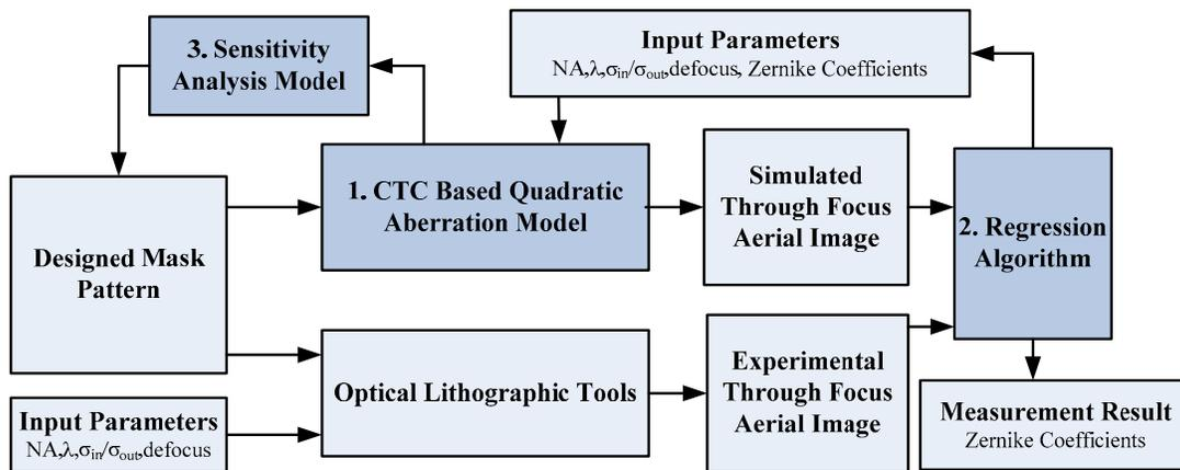
Fig.1. The flowchart of the aberration measurement using the CTC-based quadratic aberration model. The Zernike coefficients are extracted by the regression algorithm from the experimental through focus aerial images.
