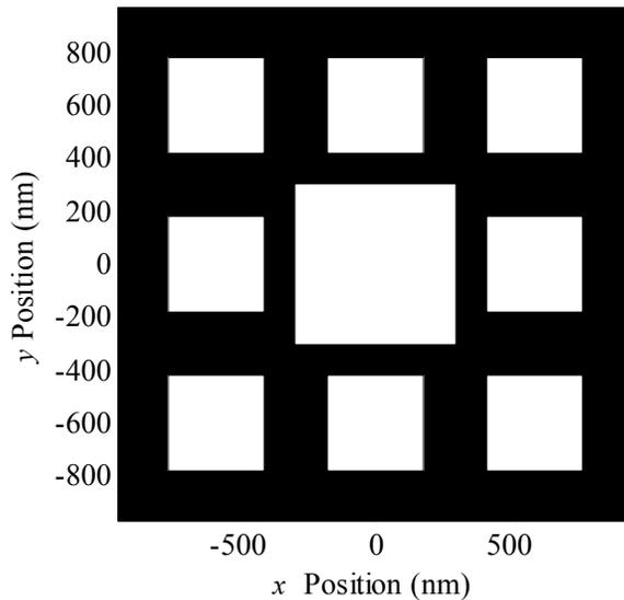
Fig. 2. The test mask pattern in aberration measurement
