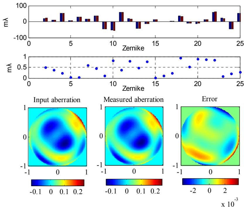
Fig. 6. Simulation result of aberration measurement for Zernike coefficients up to 25th order.
