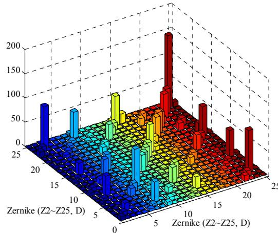
Fig. 5. The average intensity of quadratic aerial image terms for Zernike coefficients up to 25th order
