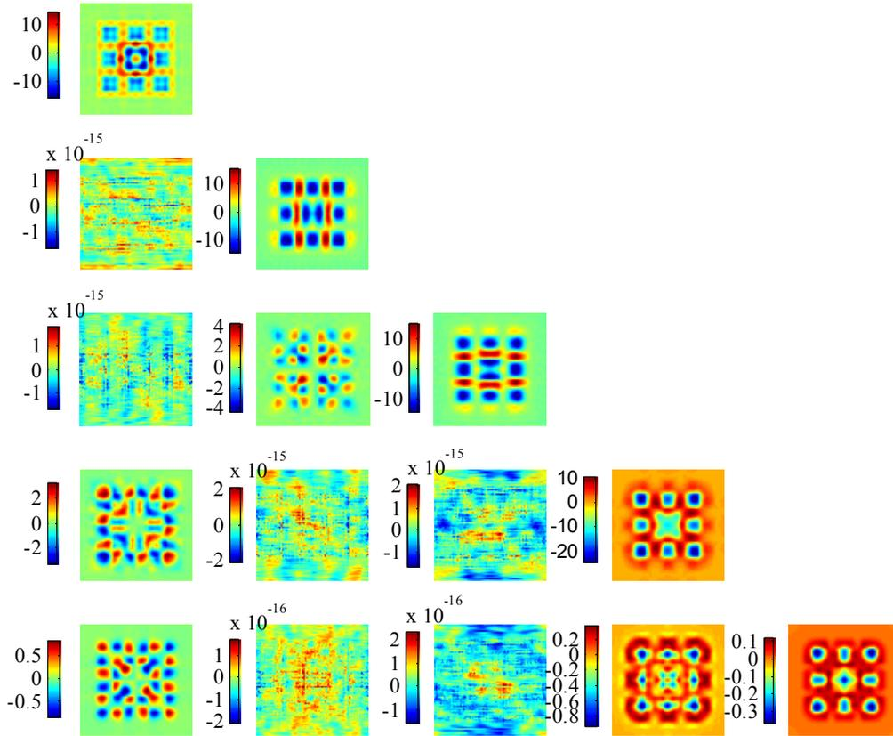
Fig. 4. The quadratic aerial image terms for Z6, Z7, Z8, Z9, and defocus, and their interaction terms. The  $x$ -axis and  $y$ -axis is  $x$  Position, and  $y$  Position for the aerial image term, and their range is  $[-1287\text{nm}, 1287\text{nm}]$ . The first column is the 6th order Zernike interact with all others, namely  $I_{\text{quad}}^{(6,6)}(\mathbf{x})$  to  $I_{\text{quad}}^{(6,D)}(\mathbf{x})$ , the then the 7th~9th Zernike to defocus in the following column.
