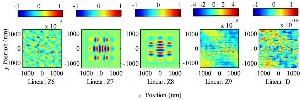
Fig. 3. The linear aerial image terms for Z6, Z7, Z8, Z9, and defocus.
