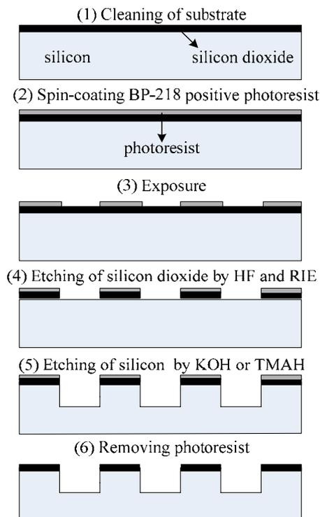
Figure 5. Schematic of the process flow etching pits in substrate
