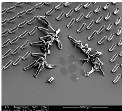
Figure 7. Collapse of high-aspect-ratio carbon microstructure prepared by C-MEMS without micromechanical interlocking
