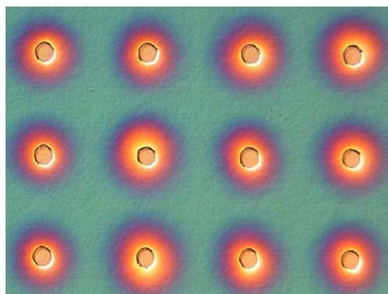
Figure 6. The pits in substrate to form micromechanical interlocking
