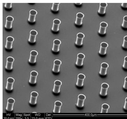
Figure 8. Straight high-aspect-ratio carbon microstructure prepared by C-MEMS with micromechanical interlocking
