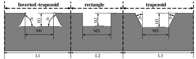
Figure 4. Cross-section schematic of the irregularity of the substrate surface
