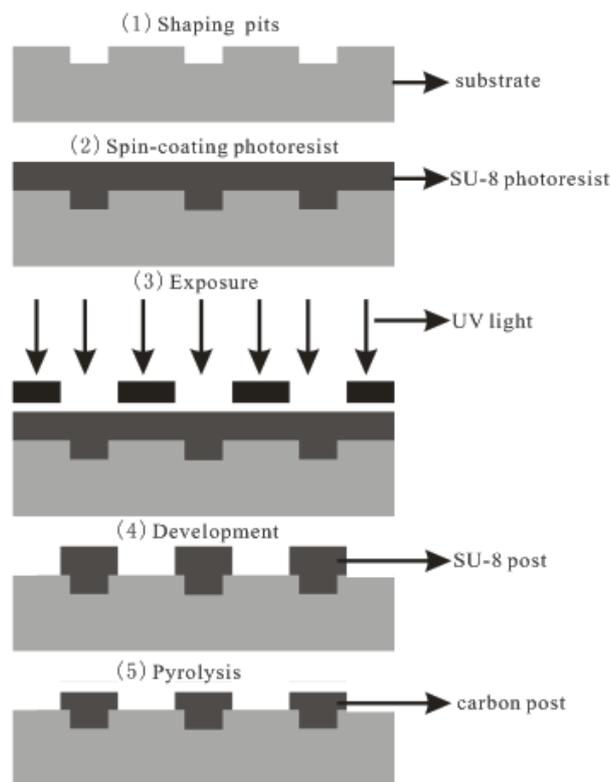
Figure 1. Schematic of the improved C-MEMS process flow
