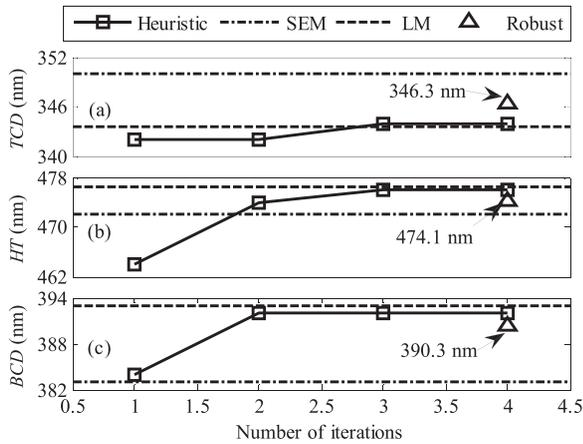
FIG. 6. Values of (a) *TCD*, (b) *HT*, and (c) *BCD* obtained by the heuristic search, the robust correction, the SEM, and LM, respectively.
