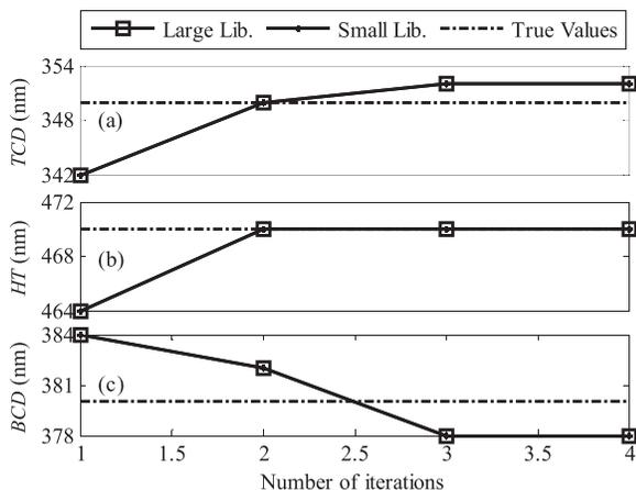
FIG. 3. Iterative values of (a)  $TCD$ , (b)  $HT$ , and (c)  $BCD$  in the heuristic search procedure for the large and small libraries, respectively.TABLE II. Extracted values of  $TCD$ ,  $HT$ , and  $BCD$  by different methods, respectively.
