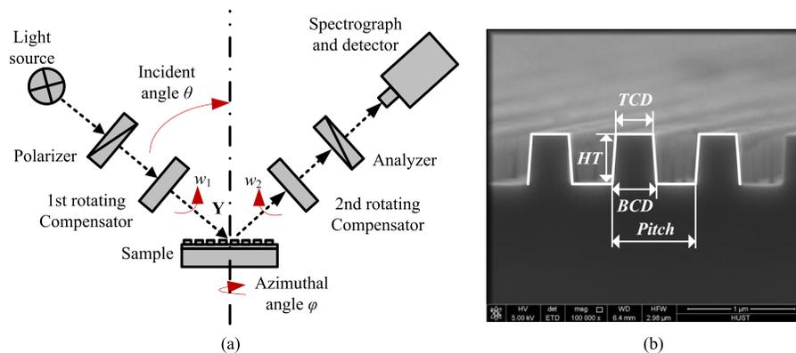
Fig. 2. (Color online) (a) Measurement setup of dual-rotating-compensator ellipsometer and (b) cross-section SEM image of one-dimensional trapezoidal etched silicon grating.
