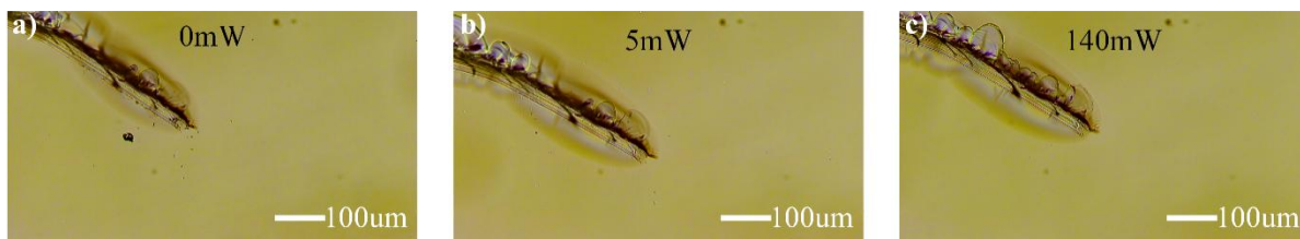
Figure S1. Direct CW laser writing on an ITO thin film without electrochemical assistance. As can be observed, it cannot generate any patterns at laser powers of a) 0 mW, b) 5 mW, and even c) 140 mW. Diamond pen scratches were used solely to locate the position. These results indicate that ITO thin film cannot be directly patterned by CW laser with power below 140 mW.
